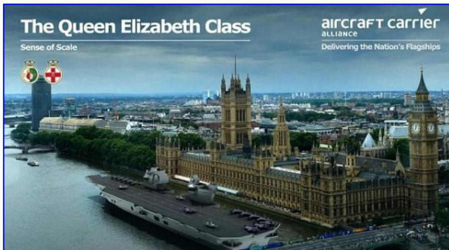
Sense of Scale. Computer generated picture of the 280m vessel in front of the 265m frontage of the Houses of Parliament—it couldn't get under the bridges!
